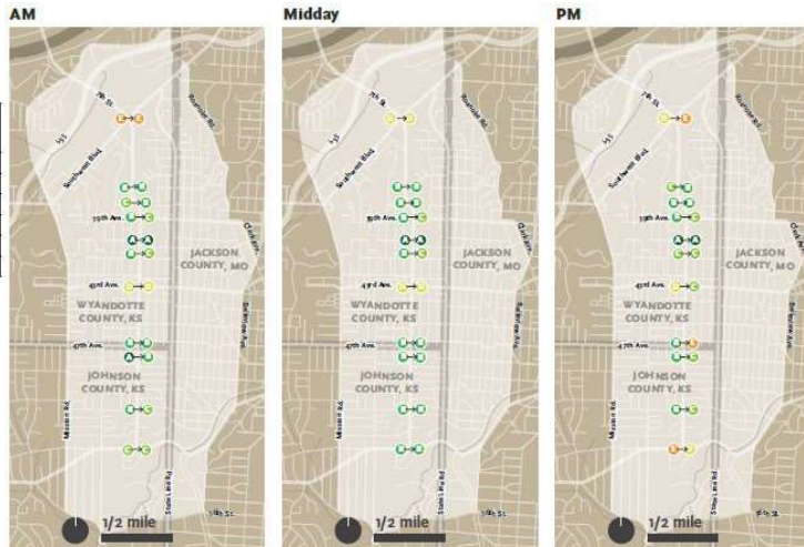
Figure 49. Change in Level of Service at AM, Midday, and PM Periods Due to a Road Diet on Rainbow Boulevard
