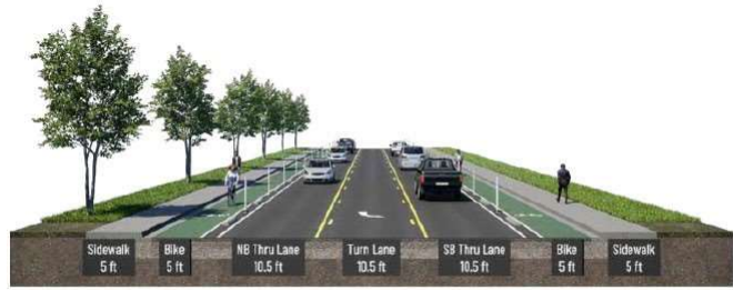
Figure 57. On-Street Bicycle Facilities South of 39th Avenue
