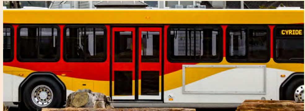
Figure 21. Large center doors on low-floor diesel bus (Source: Gillig)
