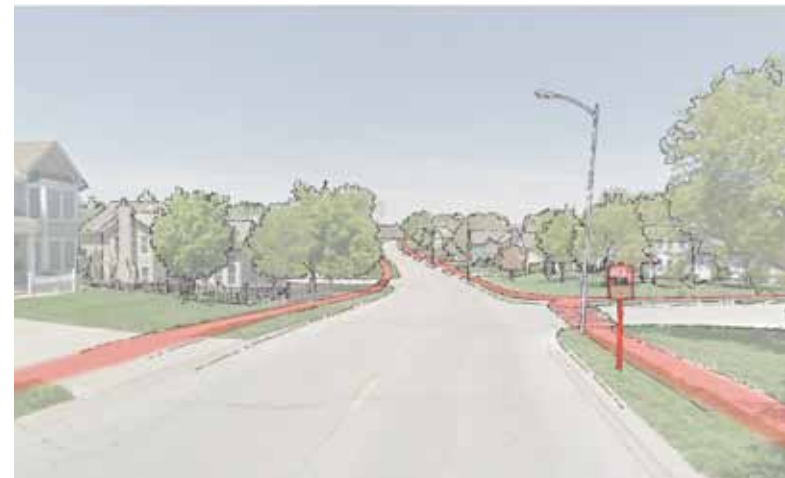
DETAIL IMAGE -S Example of widened sidewalks and added signage with an existing neighborhood
